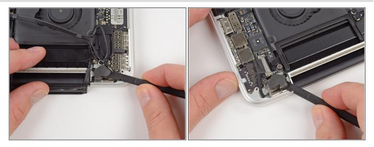
• Use the flat end of a spudger to pry the rubber hinge covers up off the left and right hinges.
